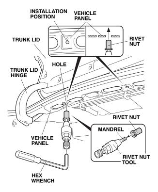
2. Open the trunk. Insert the rivet nut into the hole in the vehicle panel, and install the hex wrench on the rivet nut tool.
